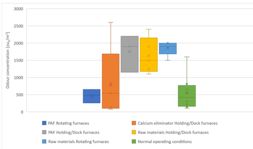
Figure 2. Box plots of odour concentration ranges of point emissions associated to different operating conditions
