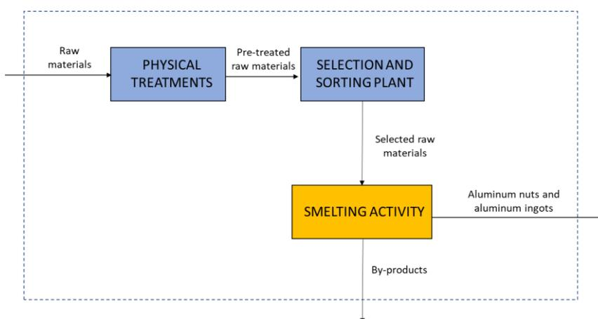
Figure 1. Scheme of the main activities carried out in the plant: pre-treatment line (blue boxes) and smelting line (yellow box)
