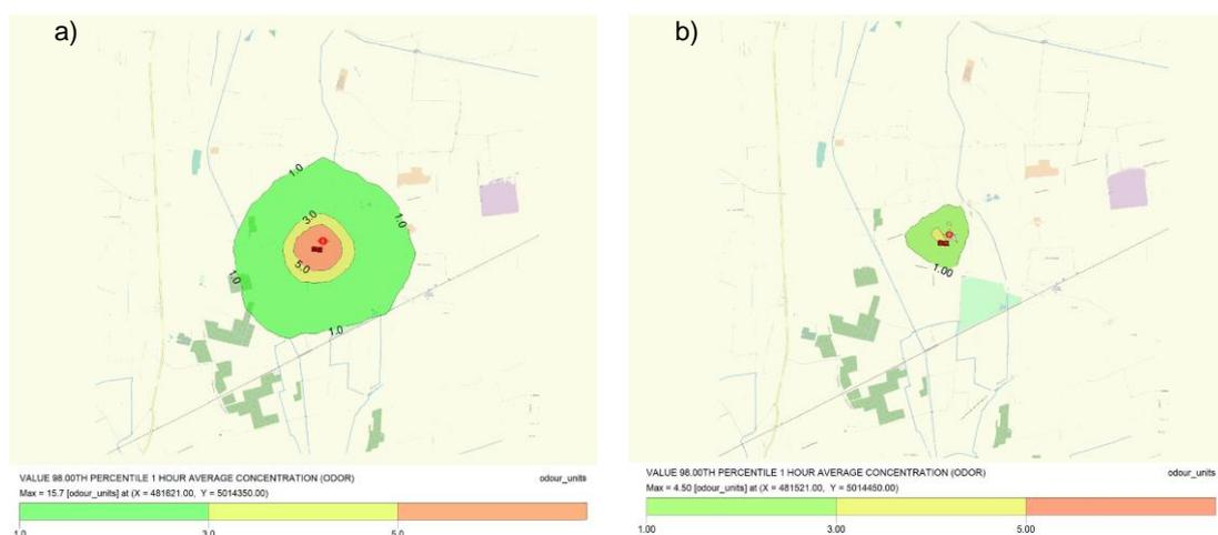
Figure 4. 98<sup>th</sup> percentile impact maps considering only diffuse emissions (a) and only point emissions (b)
