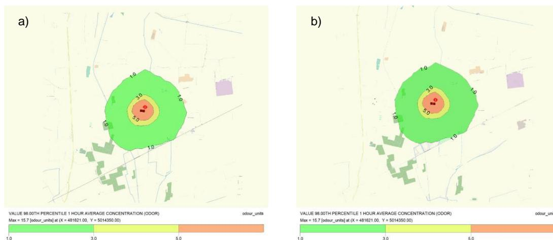
Figure 3. 98<sup>th</sup> percentile impact maps corresponding to two different randomizations of the dispersion model
