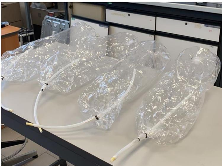
Figure 1. Example of the sampling collection bags with the gas samples used in this study.
