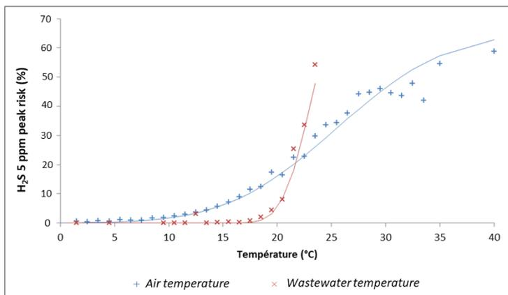
Figure 1: Risk of a 5 ppm H<sub>2</sub>S peak at SAV depending on air and water temperature
