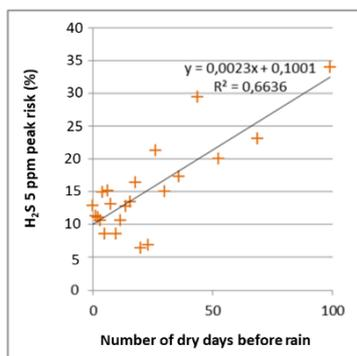
Figure 4: Risk of a 5 ppm H<sub>2</sub>S peak at SAV depending on the number of dry days before rain
