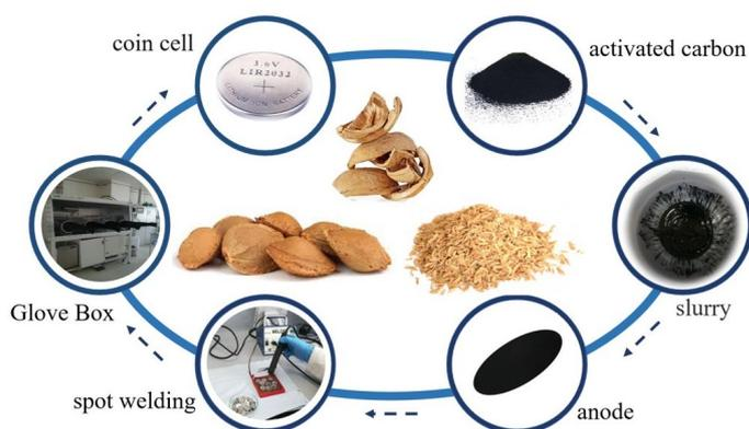
Figure 1. The schematic diagram for the creation of coin cell
