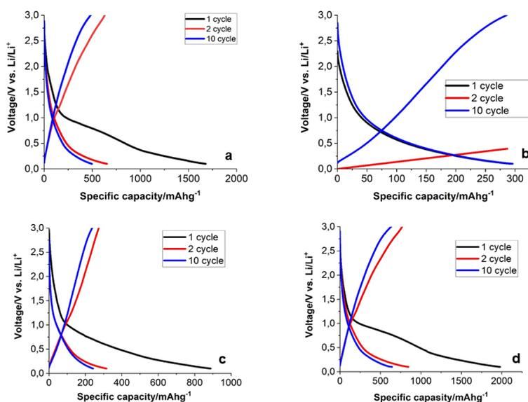
Figure 3. Charge-discharge profiles of batteries with carbon electrodes: (a) apricot stones; (b) rice husk 1; (c) rice husk 2; (d) walnut shell
