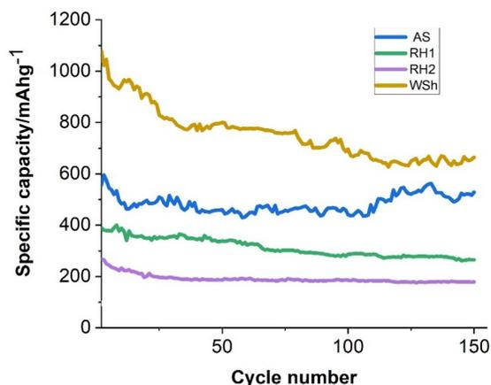
Figure 4. The cycling performance of batteries with obtained carbon electrodes
