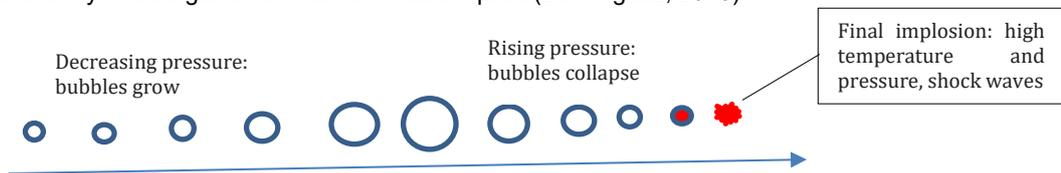
Figure 1. Growth and collapse of a bubble by hydrodynamic cavitation (García and Calvo, 2013)
