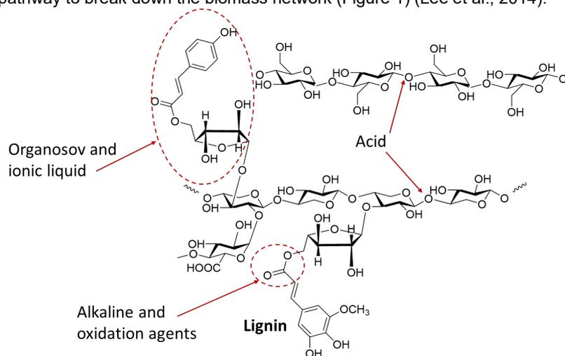
Figure 1: The attack of different agents on the lignocellulosic structure.
