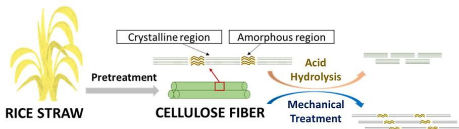
Figure 2: The acid hydrolysis and mechanical treatment of rice straw fibers
