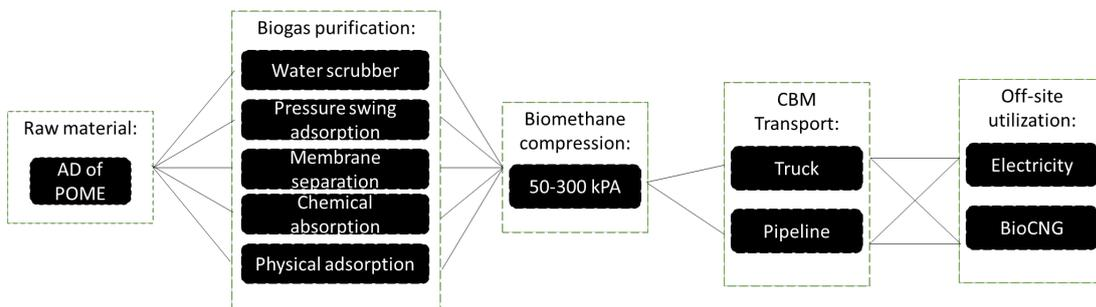
Figure 1: POME to biomethane off-site utilisation superstructure
