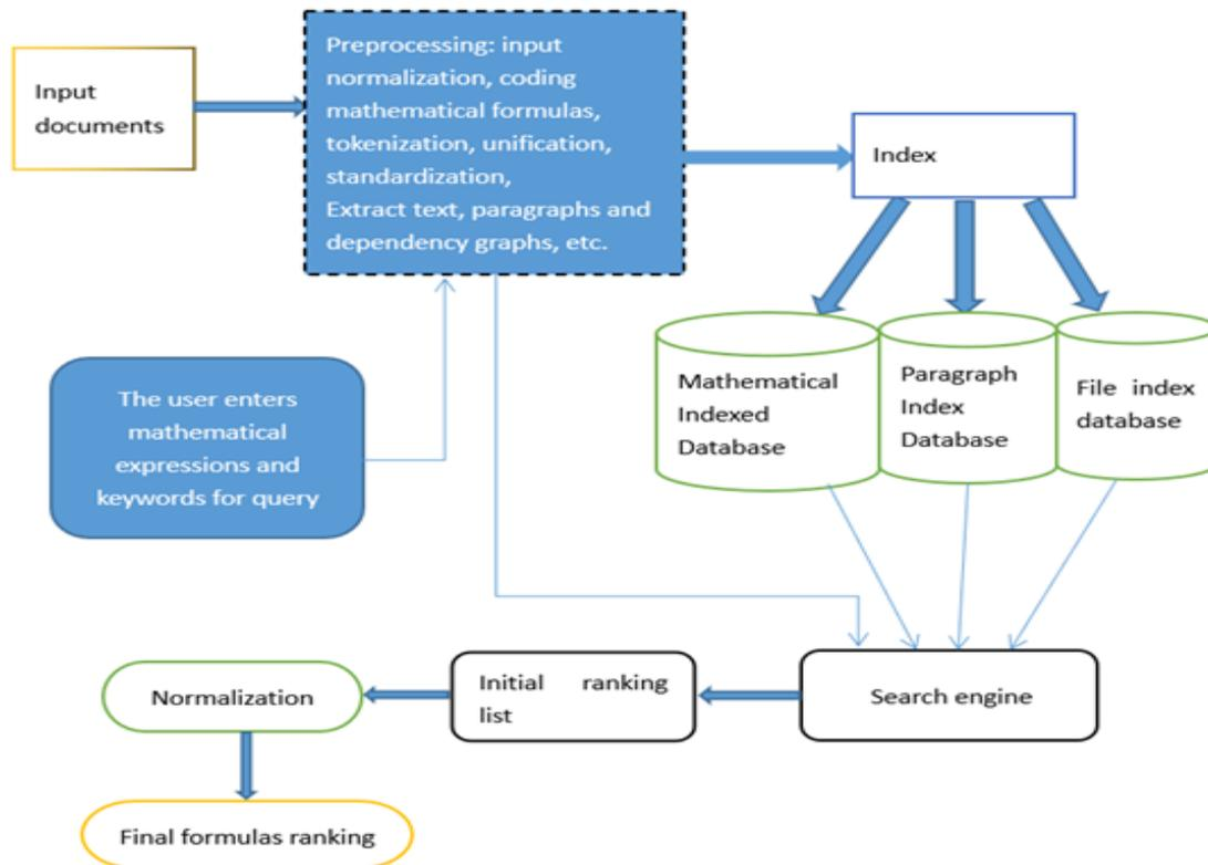
Figure 1. The overall architecture of the system
