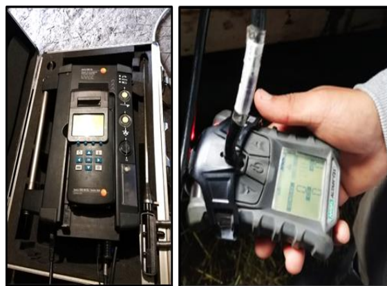
Figure 5: Gas measurement equipment TESTO X-350 y ALTAIR 4X
