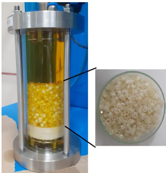
Figure 1: Hydrogel bed for removal of water from fuels
