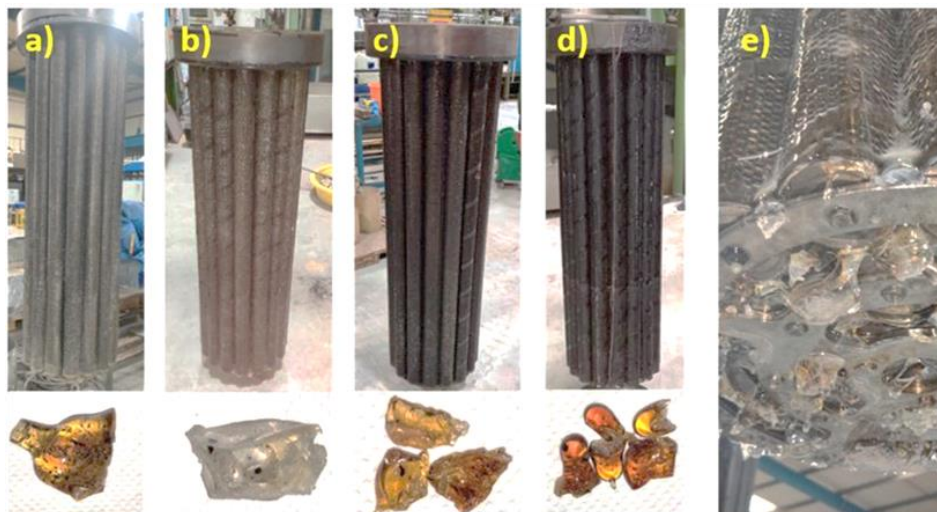
Figure 2: Filters contaminated with PET and other materials a) F14, b) F15, c) F16, d) F19, e) F15 close-up
