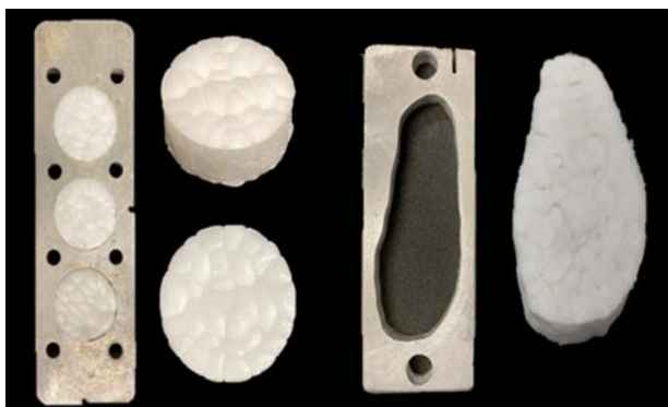
Figure 2. Molds used for the graded foaming experiments (cylindrical, top; shoe midsole bottom) and samples obtained thereof.
