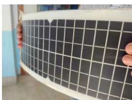
Figure 1: Thin, light and able to flex Solar panel, 0.40 m x 0.16 m, 10 W, 5V/12-18V, price 30 euro.
