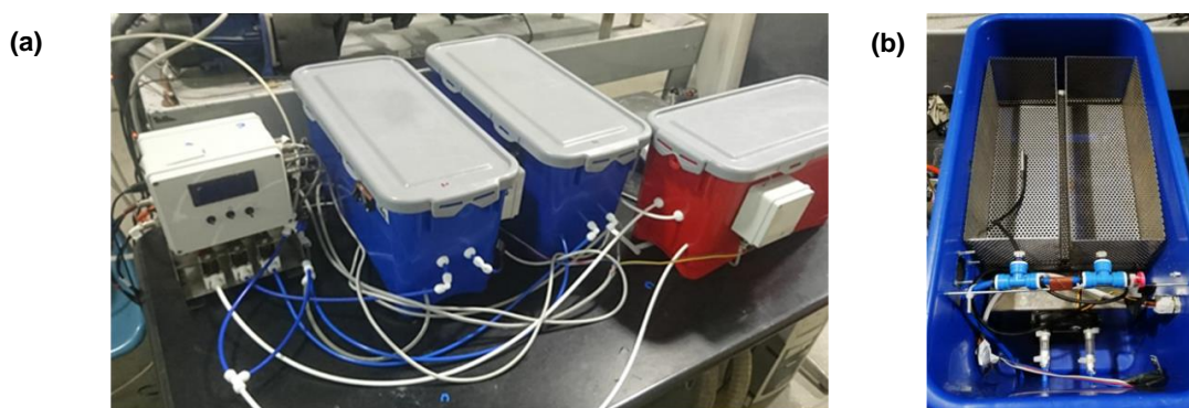
Figure 2: Pictures of the bench-top plant used in this work: (a) insulated chamber and (b) perforated baskets.
