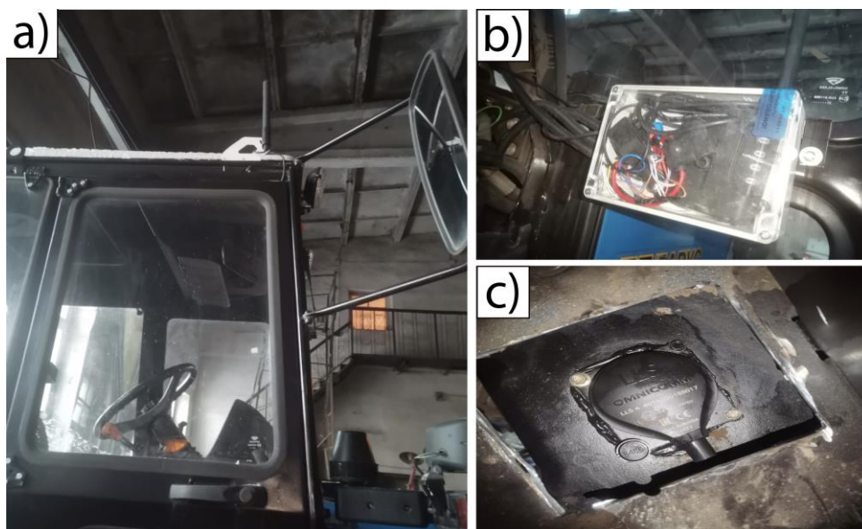
Figure 6: Installed tracker equipment kit a) GSM amplifier antenna; b) Tracker terminal; c) Fuel level sensor
