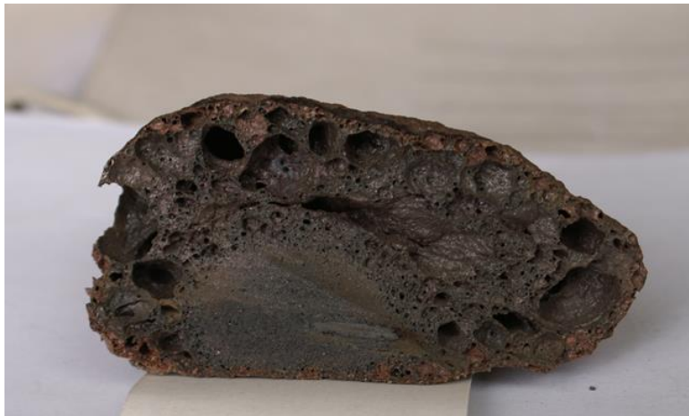
Figure 4: A sample of aluminosilicate material prepared using an ash fraction larger than 300 \mu\text{m}
