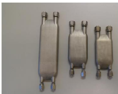
Figure 3. 3D printed reactors used as heat exchangers and reactors within the study.
