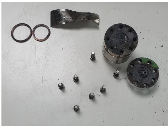
Figure 7: Photograph of the pressure transducer affected by the loss of containment at 100 bar at 235 °C.
