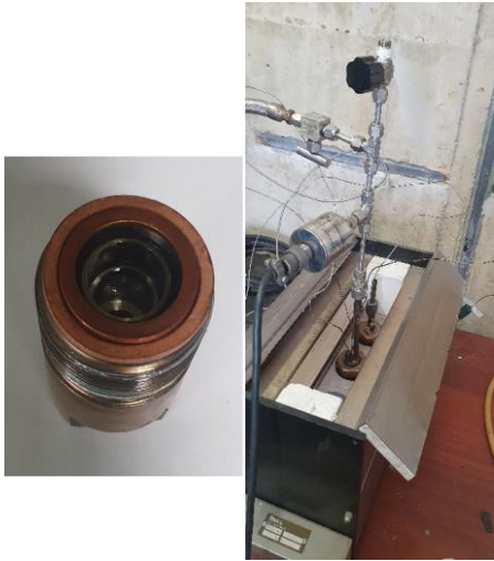
Figure 4. Photograph of a setup assembly a) 5 g Acetonitrile in glass tube, b) Mini-autoclave set-up inside heating block.
