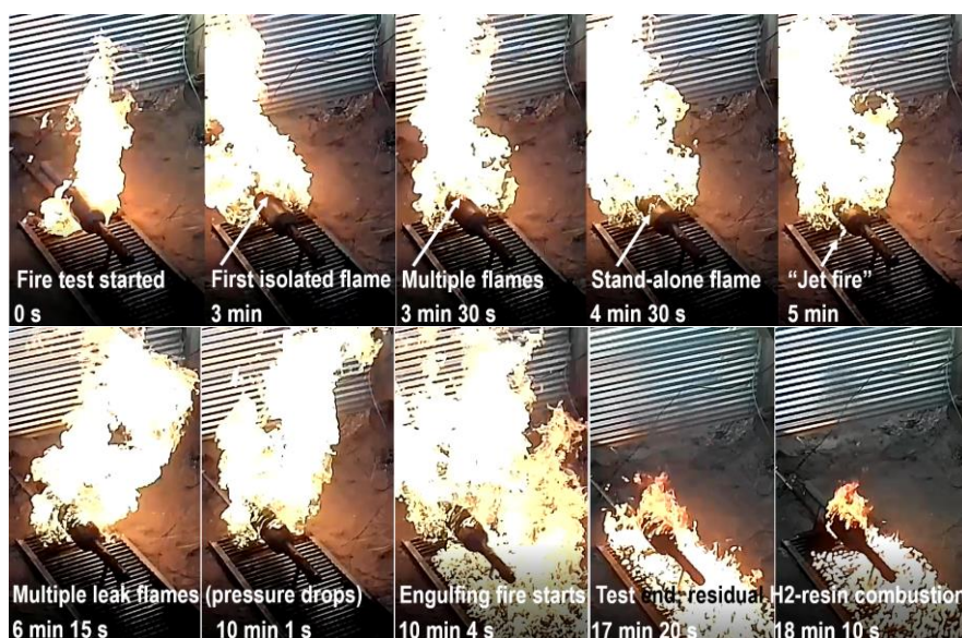
Figure 5: Snapshots of one of \mu LNB tank prototypes behaviour in a fire test with realistic HRR/A=1 \text{ MW/m}^2
