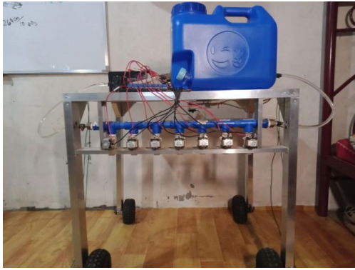
Figure 5: The smart weed control system
