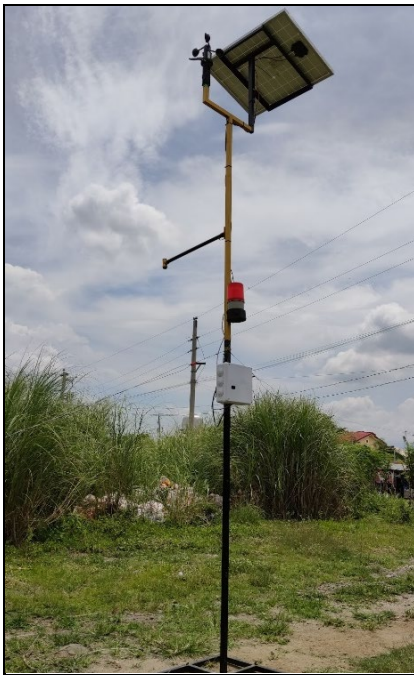
Figure 2: Actual fabricated prototype of the weather station
