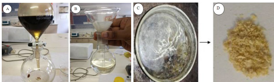
Figure 1: Image of (a) liquid-liquid extraction of caffeine and solvent, (b) organic phase containing caffeine, (c) extracted crude caffeine and (d) extracted powder caffeine
