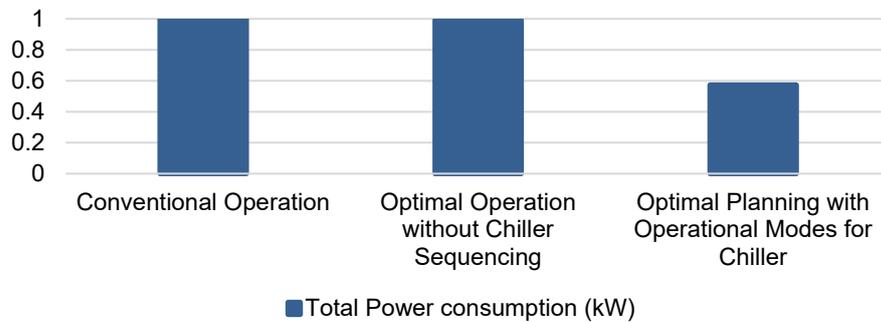
Figure 3: Total power consumption for alternative operations of multi-compressors refrigeration system
