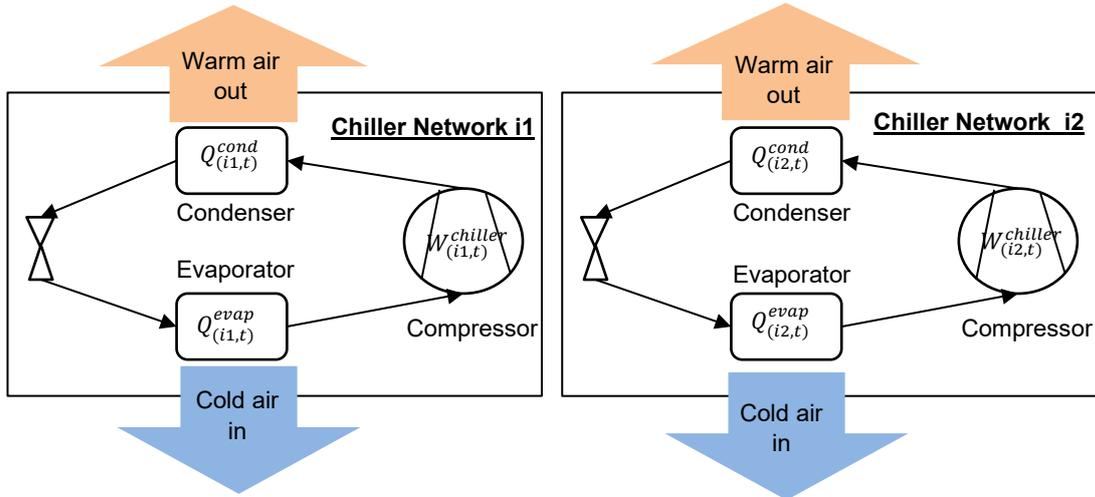
Figure 1: Chillers network in parallel for vapour compression refrigeration system
