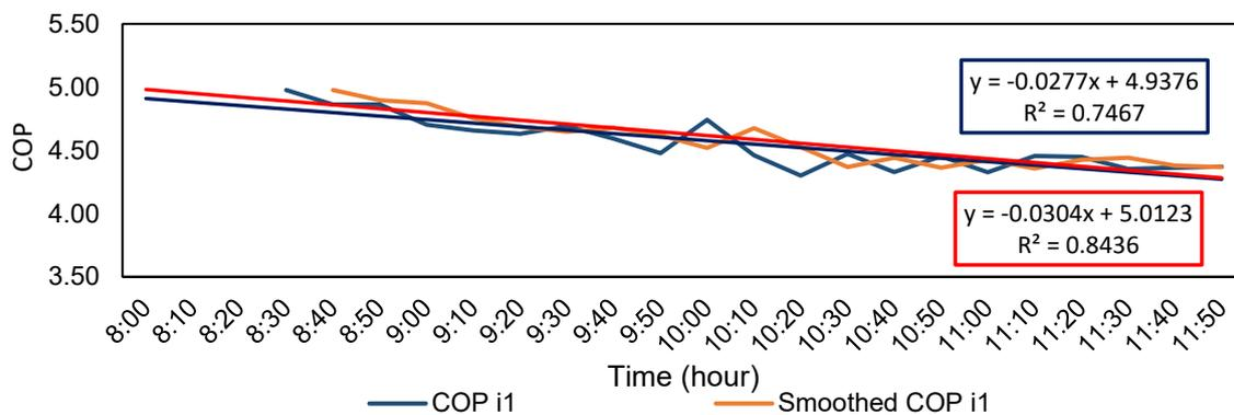
Figure 4: Optimal time-varying COP profiles for compressor i1 of chillers network
