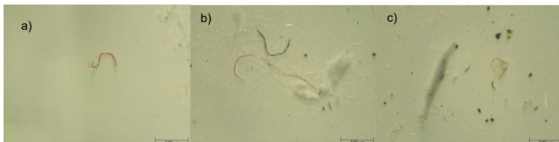
Figure 2: The stereomicroscope image of microplastic with (a) fiber shape (b) long fiber shape and (c) fragment shape
