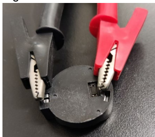
Figure 2: Connection of coil cell holder and the potentiostat
