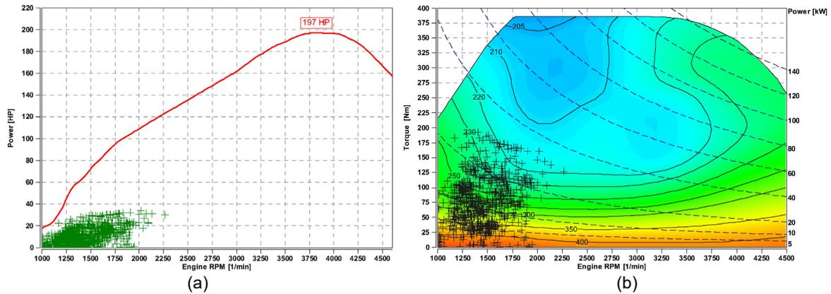
Figure 2 (a) BSFC [g/kWh] according to torque with urban working points, (b) Power curve of the car with urban working points
