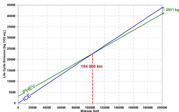
Figure 3: Life Cycle Assessment of the conventional and plug-in hybrid drivetrain
