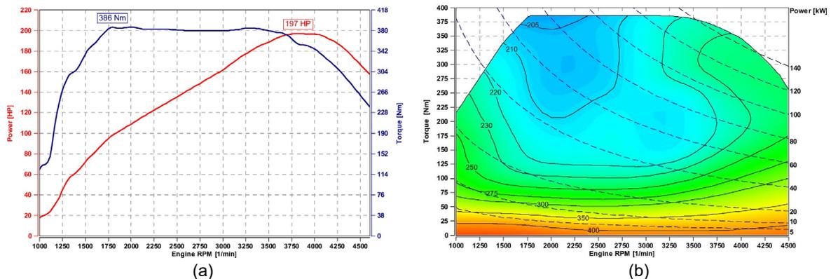
Figure 1: (a) Power and torque curves of the investigated car regarding OBD measurements, (b) BSFC [g/kWh] according to torque
