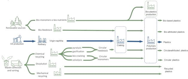
Figure 4: Traditional and new plastic production chains
