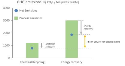
Figure 5: End-of-life processes comparison (adapted from ChemCyclingTM: Enviromental Evaluation by Life Cycle Assessment, BASF, 2020)
