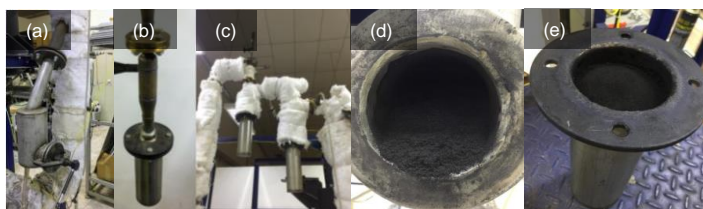
Figure 1: (a) Biochar 1 reservoir coupled to the reactor; (b) Cyclone with the respective reservoir without coating; (c) Biochar 2 and Biochar 3 reservoirs (from right to left – Biochar 1 is right below in the left of the figure); (d) First biochar reservoir (Biochar 1); (e) Representation of 2 nd and 3 rd biochar reservoirs (they are similar)
