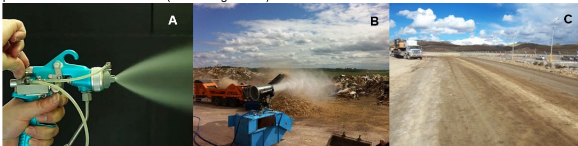
Figure 3: A) Spray gun. B) Dry fog application. C) Treated area.
