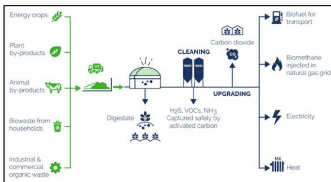
Figure 2: Plant scheme for biogas
