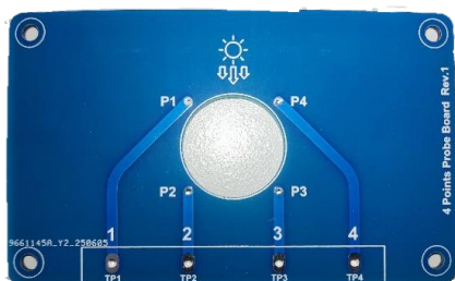
Figure 1a: Top panel of the custom-built experimental setup for four-point probe measurements.
