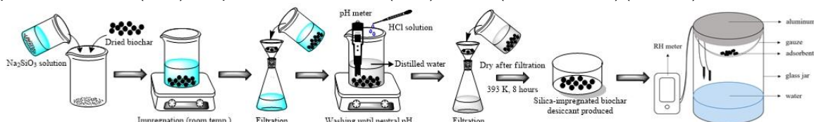
Figure 1. The preparation process and experimental setup of biochar based composite desiccant
