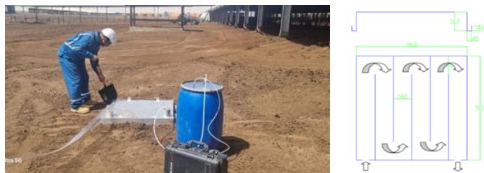
Figure 2: Image of Lindvall hood sampling system being place within a paddock area and a schematic image showing the dimensions of the Lindvall hood
