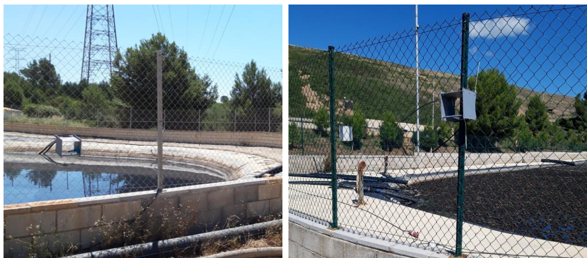
Figure 1: Leachate basin. H 2 S sampling during July 2020 (left) and September 2025 (right) campaigns.
