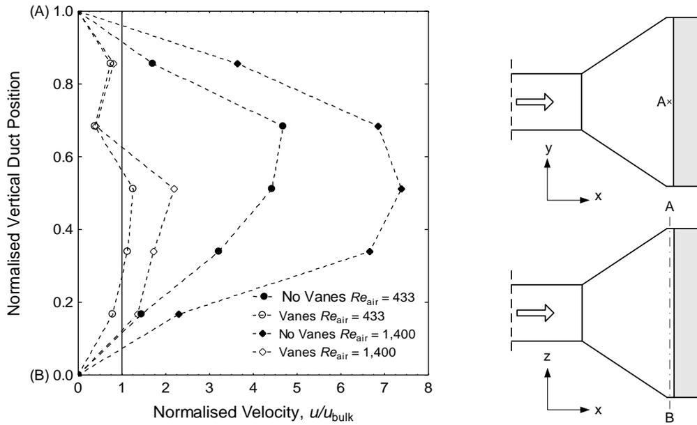
Figure 2: Normalised velocity profiles at the end of the diffuser directly prior to the heat exchanger along vertical line AB with and without flow correction vanes at two different air-side Reynolds numbers
