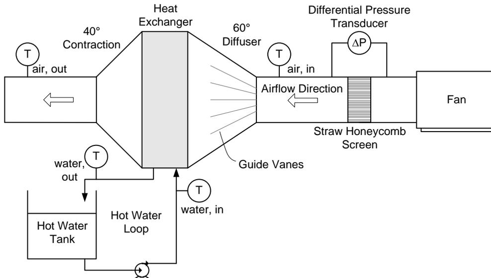
Figure 1: Schematic of the experiment heat exchanger rig (not to scale)
