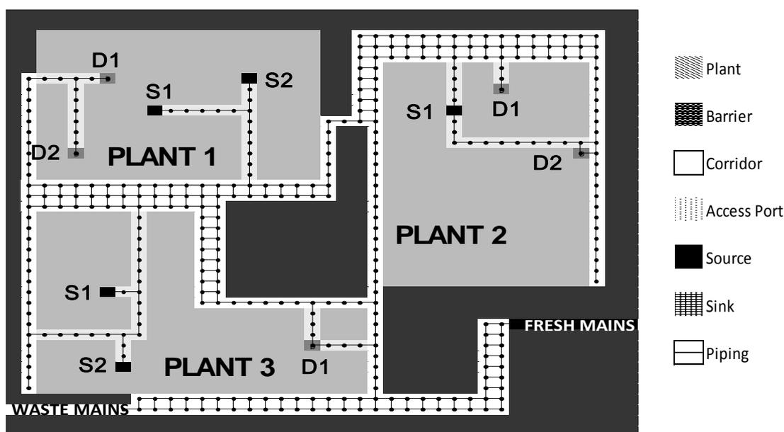
Figure 1: Industrial city layout illustrated using Type 1 piping connectivity
