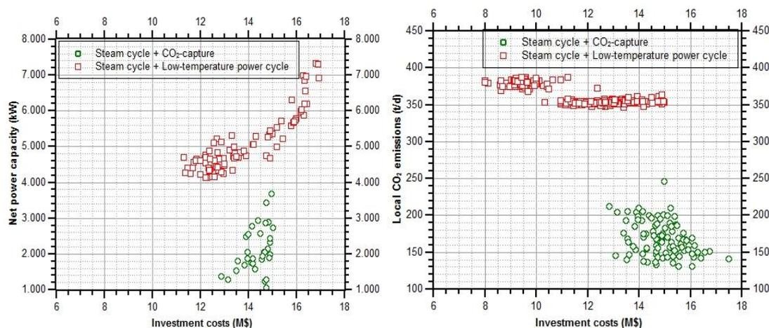
Figure 4: Thermo-economic and thermo-environmental Pareto frontiers comparing the maximum power capacity (left) and the CO<sub>2</sub>-reduction potential (right) against the total investment cost
