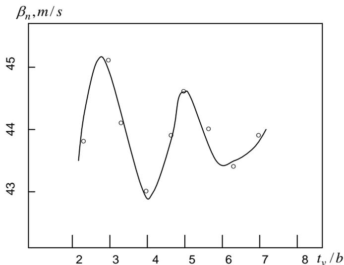
Figure 1: The dependence of mass transfer coefficient on the dimensionless vertical step between turbulence induced units. Gas velocity  $W_g = 15$  m/s; horizontal step  $t_h = 2b$
