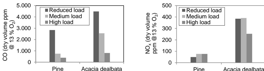
Figure 3: CO and NO<sub>x</sub> emissions for Pine and Acacia pellets at reduced, medium and high loads
