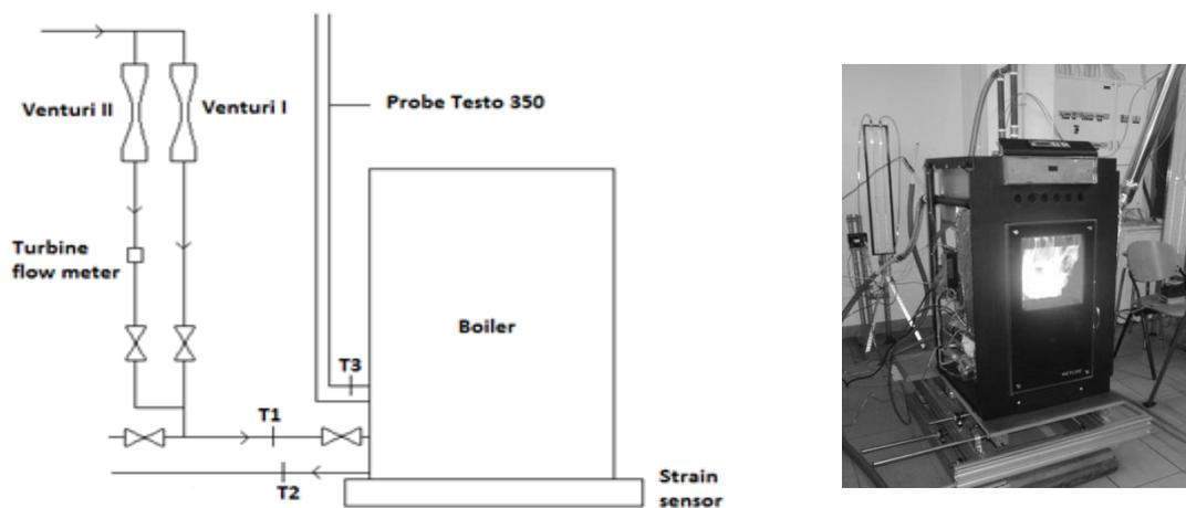
Figure 1: Experimental set-up (scheme and photo) Performance measurements
