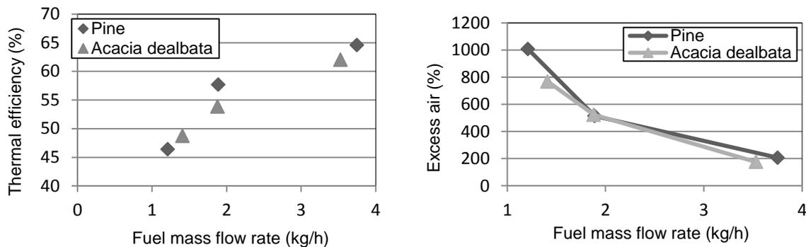
Figure 2: Thermal efficiency and excess air as a function of fuel mass flow rate
