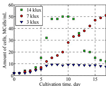
Figure 4: Dynamics of biomass growth in Tamiya medium at different levels of illuminance
