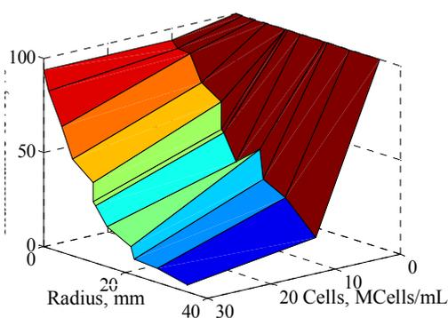
Figure 6: Dependency of illuminance level on the radius and the concentration of cells
