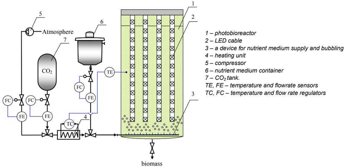
Figure 1: Basic diagram of a laboratory unit for the cultivation of microalgae biomass
