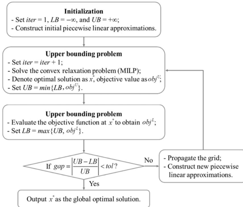
Figure 2. Flowchart of the successive piecewise approximation algorithm
