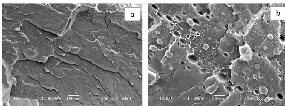
Figure 1: SEM micrographs of fracture surface of PE (a) and HC/PE blend at 20 wt% HC (b).
