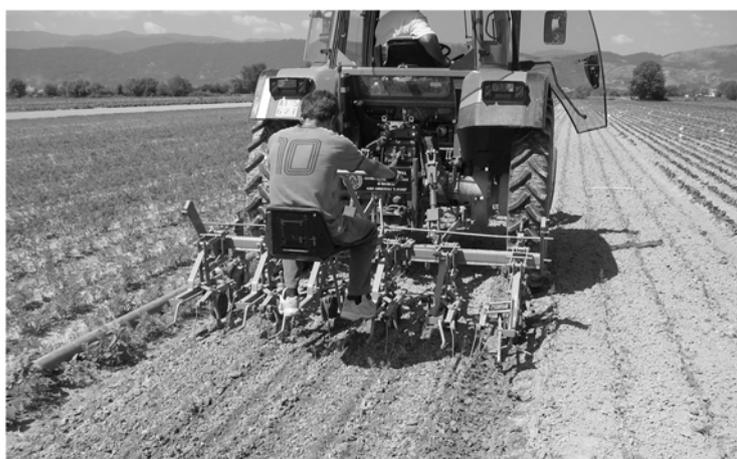
*Figure 3: Precision hoe at work in fennel*
