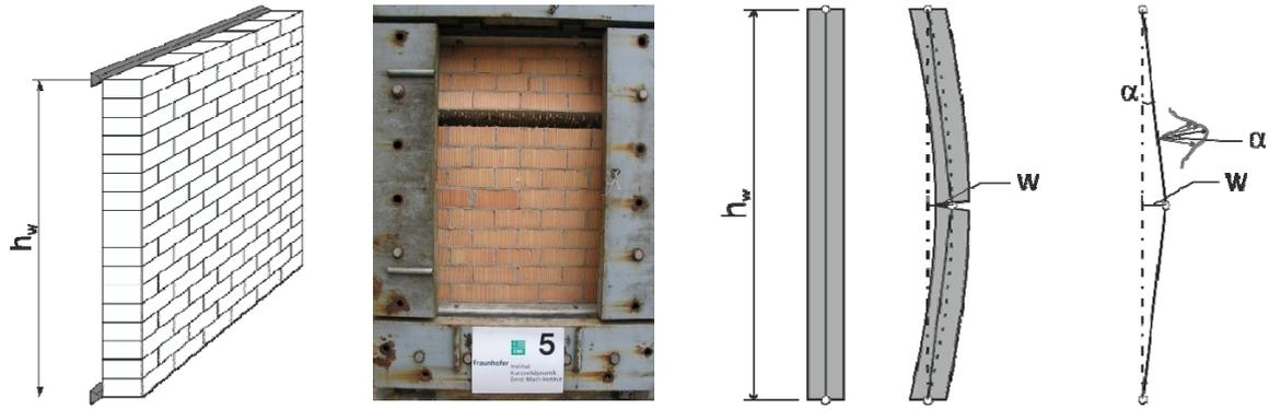
Figure 1: Left, single-span wall system. Center, single-span wall system at the onset of the break-up process. Right, two-dimensional mechanical model at ultimate and fragment launch angle distribution.
