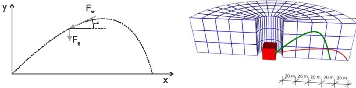
Figure 2: Left, Trajectory of a single fragment indicating gravity and air drag. Right, Exemplary discretization of the spatial surroundings to monitor flight trajectories (Dörr et al., 2002).
