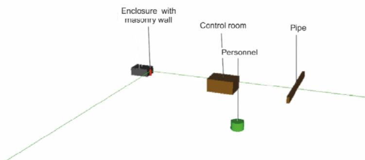
Figure 3: Exemplary scenario showing the masonry wall (debris source) and surrounding components.
