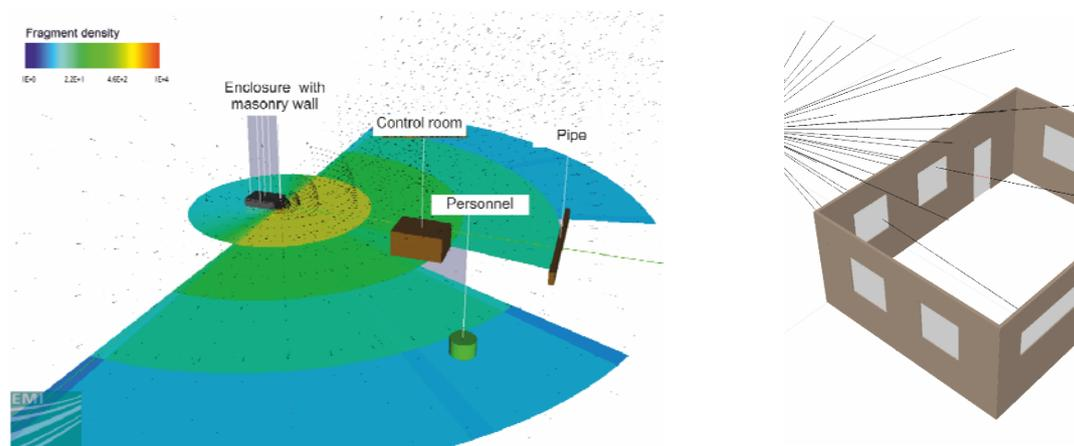
Figure 4: Left, fragment density with  $E \geq 79$  J on ground after exemplary wall break-up. Right, penetration of structural components of the "control room" by critical fragments originating from the masonry wall.
