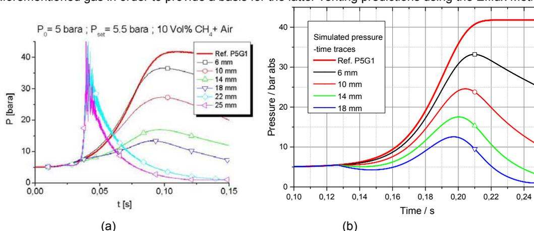
Figure 1: Influence of the venting diameter on the pressure profiles of a vented 6 l autoclave without obstacles (a) (Poli 2013) and pressure time traces simulated using the Efflux Method (b),  $A_T = 1$ .
