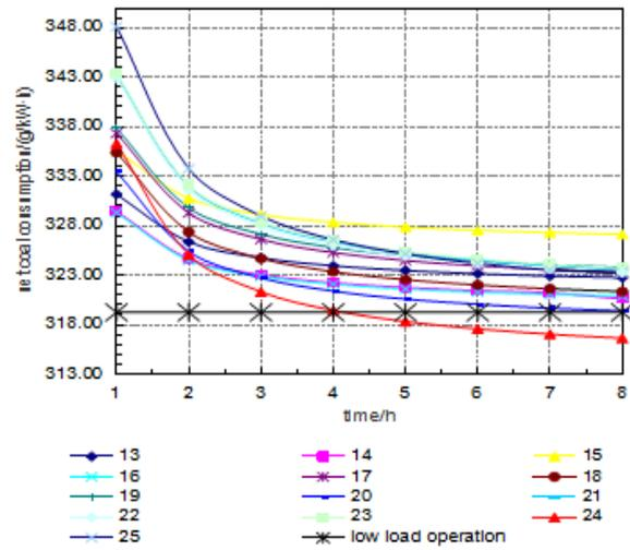
Figure 2: Peak coal consumption curve of 600MW
