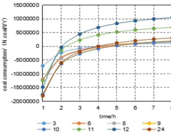
Figure 3: Comparison of coal conservation and emission reduction for different peak load regulation schemes (for 70% capacity of pumped storage units)
