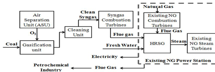
Figure 3: Revamped natural gas combined cycle power plant
