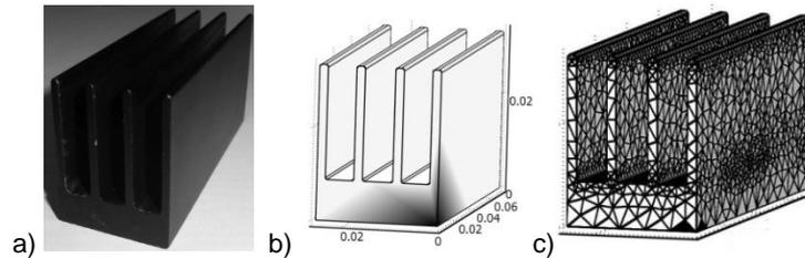
Figure 1: Geometry of the modelled device: a) view of the real object b) 3-D model c) FEM mesh
