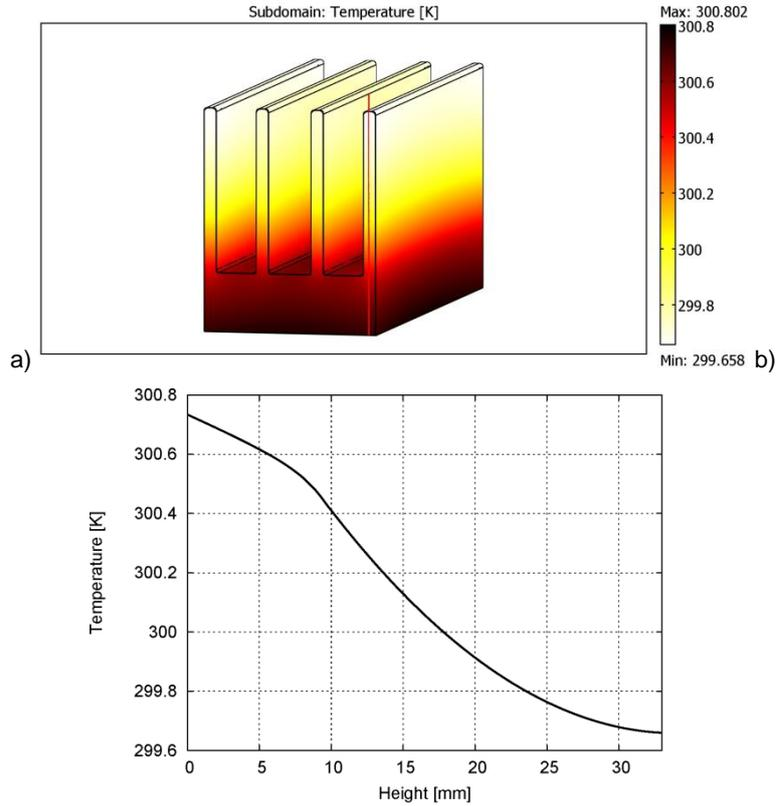
Figure 3: Temperature distribution: a) at the radiator surface, b) along the radiator height
