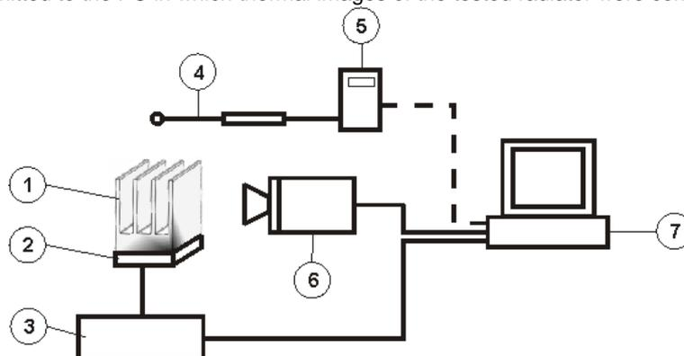
Figure 2: Scheme of the measurement stand. Markings: 1 Radiator, 2 Heater, 3 High current amplifier, 4 Probe, 5 Anemometer, 6 Thermovision camera, 7 PC. The dashed line - manual transfer of information
