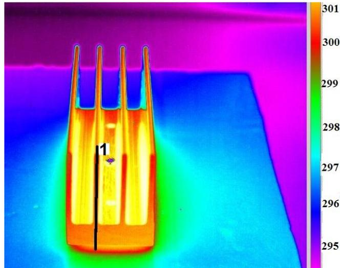
Figure 4: Thermogram of the radiator
