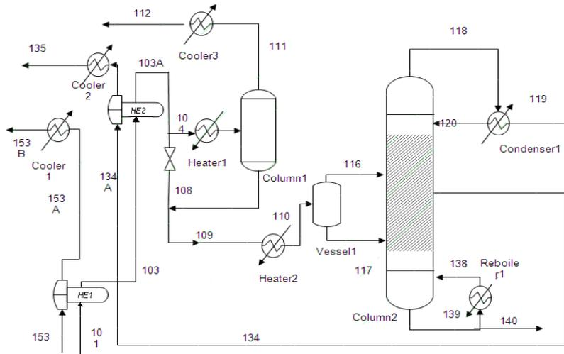
Figure 1: Heat exchanger network (HEN) for fatty acid fractionation plant (Abu Bakar et al., 2015a)
