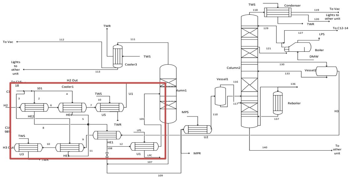
Figure 3: Process flow diagram of new HEN for a unit in FAFP
