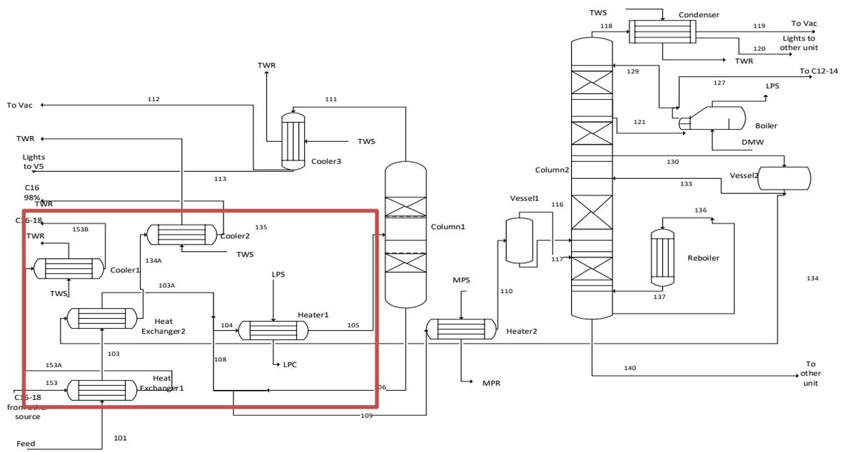
Figure 2: Process flow diagram of original HEN for a unit in FAFP
