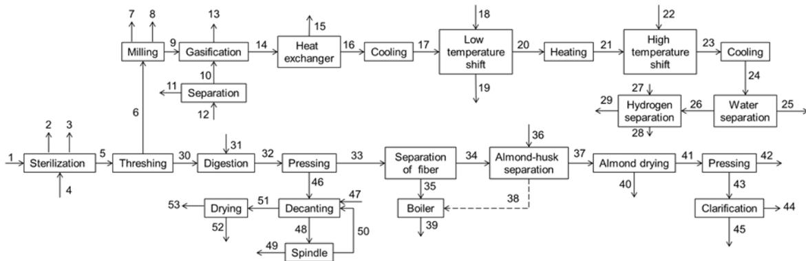
Figure 1: Topology of palm fruit-based biorefinery
