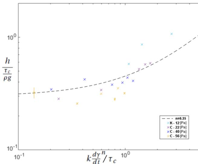
Figure 6: Dimensionless coating thickness  $h / (\tau_c / \rho g)$  plotted against the inverse of the dimensionless Bingham number. The points K-12 were obtained using the ketchup sauce, while the others were obtained using the Carbopol solutions. For all liquids, the number indicates the yield stress. The dashed line shows the prediction of the theory described in eq. 4. (Maillard et al. 2014)
